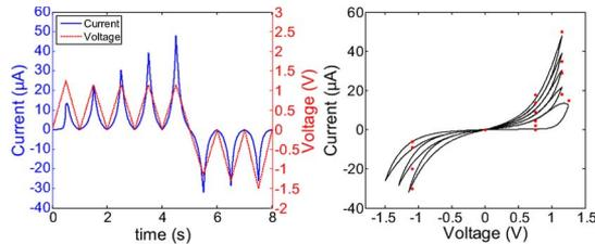
Fig. 4. Results obtained for matching characterization in [3]. Dots show the points from [3]. In this simulation,  $V_p = 0.9$  V,  $V_n = 0.2$  V,  $A_p = 0.1$ ,  $A_n = 10$ ,  $x_p = 0.15$ ,  $x_n = 0.25$ ,  $\alpha_p = 1$ ,  $\alpha_n = 4$ ,  $a_1 = 0.076$ ,  $a_2 = 0.06$ ,  $b = 3$ , and  $x_0 = 0.001$ .
