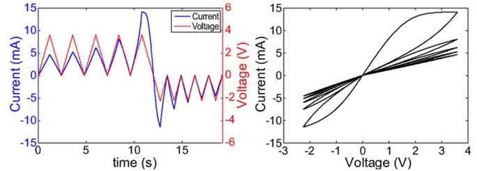
Fig. 1. Simulated  $I$ - $V$  characteristic using the memristor model in [7].
